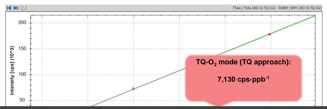
Use of O<sub>2</sub> as a reactive gas improves detection sensitivity for <sup>75</sup>As in comparison to KED
